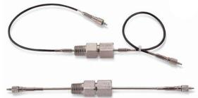
FSA optical fiber sealing assemblies enable a range of sizes of fiber optic cable to pass through environmental boundaries. Fibers are housed in individual, protective stainless steel tube seals. These may be supplied as a complete integral assembly with connectors, in one of the standard pressure and vacuum seal fittings.
