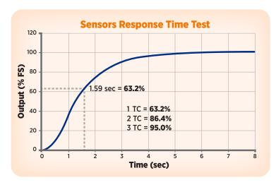
A typical speed of response curve demonstrates how quickly a particular sensor responds to changes in temperature.
